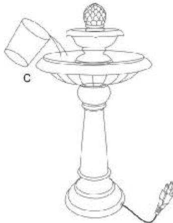
**Step 6:** Finally, connect the plug of pump (F) to a GFCI outlet.
