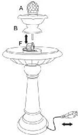
**Step 5:** Fill the basin (C) with clean water, making sure the pump (F) is fully submerged.
