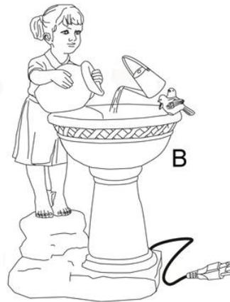
**Step 4:** Finally, connect the plug of pump (E) to a GFCI outlet.
