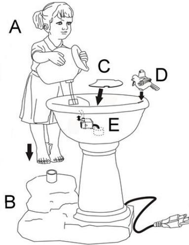
**Step 3:** Fill the basin (B) with clean water, making sure the pump (E) is fully submerged.
