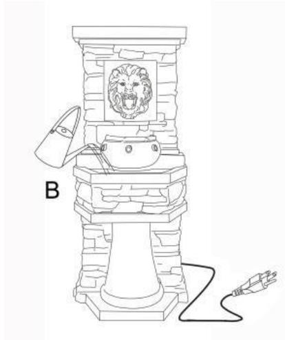
**Step 3:** Finally, connect the plug of pump (C) to a GFCI outlet.
