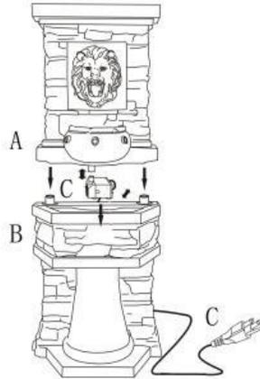
**Step 2:** Fill the basin of the bottom basin (B) with clean water, making sure the pump (C) is fully submerged.
