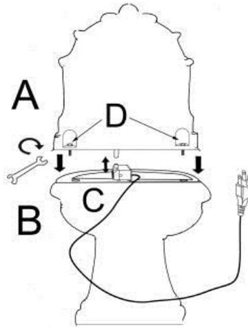
**Step 3:** Fill the basin (B) with clean water, making sure the pump (C) is fully submerged.
