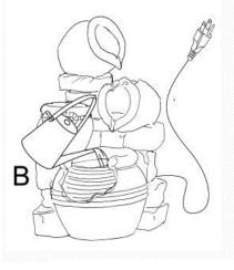
**Step 4:** Finally, connect the plug of pump (C) to a GFCI outlet. **WARNING:** Always disconnect the pump (C) before placing your hands in the water.
