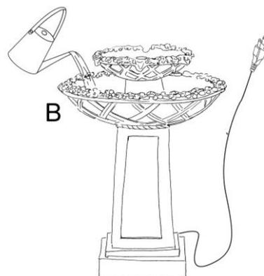
**Step 5:** Finally, connect the plug of pump (D) to a GFCI outlet.
