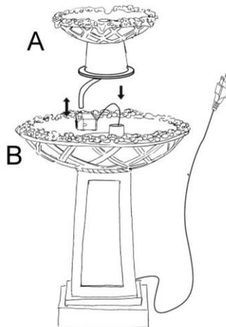
**Step 4:** Fill the basin (B) with clean water, making sure the pump (D) is fully submerged.
