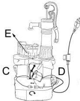
**Step 4:** Fill the basin (C) with clean water, making sure the pump (D) is fully submerged.
