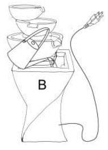
**Step 3:** Finally, connect the plug of pump (C) to a GFCI outlet.
