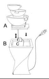
**Step 2:** Fill the basin of the bottom (B) with clean water, making sure the pump (C) is fully submerged.
