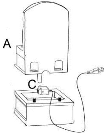
**Step 2:** Align and attach the top part (A) to the bottom (B), using the bolts and washers to fix both parts.
