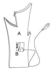
**Step 2:** Fill the basin (A) with clean water, making sure the pump (B) is fully submerged. **Note:** The maximum water level should be approximately 1.2 inches below the top edge of the basin (A).
