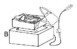
**Step 4:** Finally, connect the plug of pump (C) to a GFCI outlet. **WARNING:** Always disconnect the pump (C) before placing your hands in the water.
