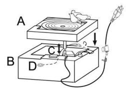
**Step 3:** Fill the basin (B) with clean water, making sure the pump (C) is fully submerged. **Note:** The maximum water level should be approximately 1.2 inches below the top edge of the basin (B).
