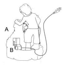
**Step 2:** Fill the basin (A) with clean water, making sure the pump (B) is fully submerged. **Note:** The maximum water level should be approximately 1.2 inches below the top edge of the basin (A).
