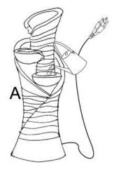
**Step 3:** Finally, connect the plug of pump (B) to a GFCI outlet. **WARNING:** Always disconnect the pump (B) before placing your hands in the water.
