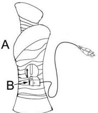
**Step 2:** Fill the basin (A) with clean water, making sure the pump (B) is fully submerged. **Note:** The maximum water level should be approximately 1.2 inches below the top edge of the basin (A).
