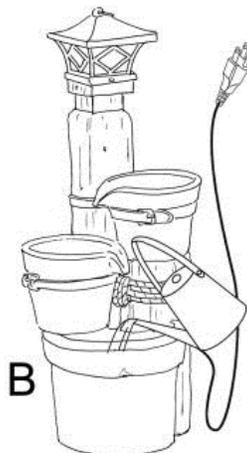
**Step 4:** Finally, connect the plug of pump (C) to a GFCI outlet.
