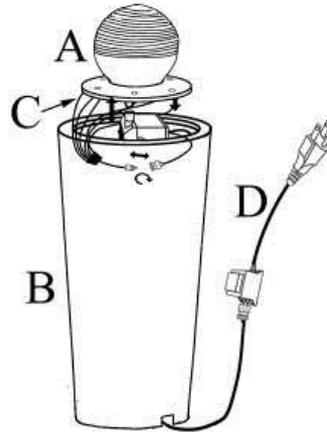
**Step 2:** Fill the base (B) with clean water, making sure the pump (D) is fully submerged
