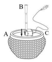
**Step 3:** Fill the bowl (A) with clean water, making sure the pump (C) is fully submerged. **Note:** The maximum water level should be approximately 1.2 inches below the top edge of the basin (A).
