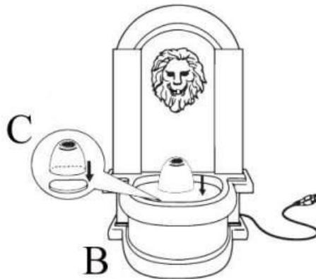
**Step 3:** Fill base (B) with clean water. Note: The maximum water level should be no higher than the water-level line on platform (C).
