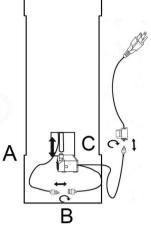
Step 2: Fill the product (A) with clean water, making sure the pump (C) is fully submerged.
