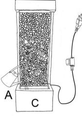
**Step 3:** Finally, connect the plug of pump (C) to a GFCI outlet. **WARNING:** Always disconnect the pump (C) before placing your hands in the water.
