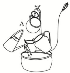
**Step 3:** Finally, connect the plug of pump (B) to a GFCI outlet.
