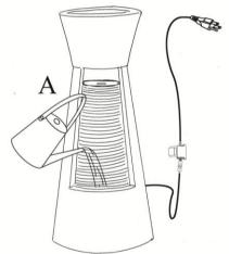
**Step 3:** Finally, connect the plug of pump (B) to a GFCI outlet. After connected, the 2 Led strips light up.
