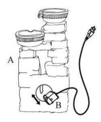
**Step 2:** Fill the basin (A) with clean water, making sure the pump (B) is fully submerged. **Note:** The maximum water level should be approximately 1.2 inches below the top edge of the basin (A).
