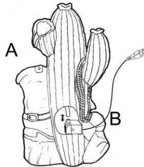
**Step 2:** Fill the boot basin (A) with clean water, making sure the pump (B) is fully submerged.
