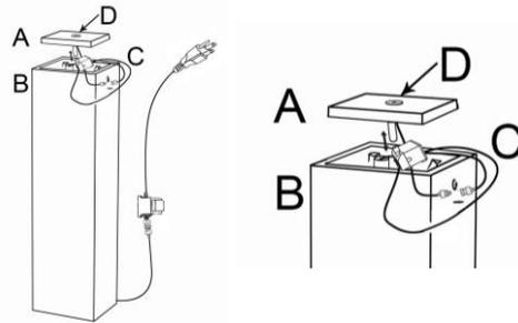
**Step 2:** Fill the basin (B) with clean water, making sure the pump (C) is fully submerged.
