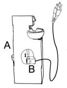
**Step 2:** Fill the bottom basin (A) with clean water, making sure the pump (B) is fully submerged.
