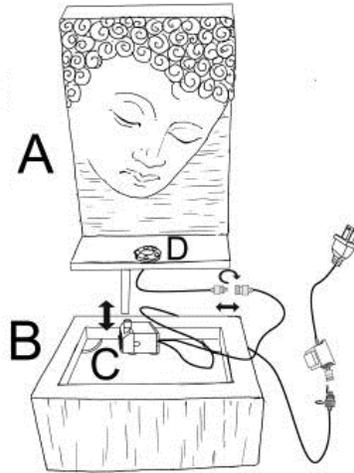
**Step 2:** Fill the basin (B) with clean water, making sure the pump (C) is fully submerged.
