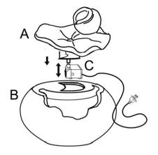
**Step 2:** Fill the plastic basin (B) with clean water, make sure the pump (C) is fully submerged.
