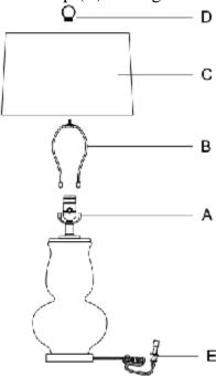
**Step 3:** Finally, connect the plug of lamp (E) to a GFCI outlet.
