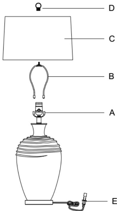
**Step 3:** Finally, connect the plug of lamp (E) to a GFCI outlet.
