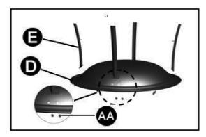
Step 3: Connect the Cross (F) to the four legs (E) using M6 Bolt (AA) and M6 Nut(BB).
