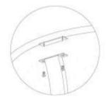
Step 3: Connect Connection Ring (E) to Leg (F) using Bolts (H). Fully tighten all bolts.
